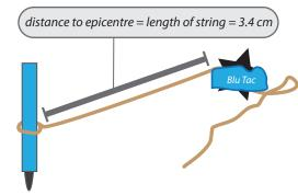
You might be asking why you need to create a compass to calculate the epicentre. This is because although you have calculated the distance from the seismometer to the epicentre, you don't know which direction it is in. By drawing a circle at the scaled distance around the seismic station, you know that the epicentre will be somewhere on the edge of the circle.
