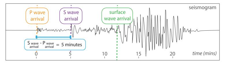
Use the example above to help you measure and record the time difference between the arrivals of the P and S wave at the three seismic recording stations (SSPA, SOCO and TEIG) on the seismogram below.
